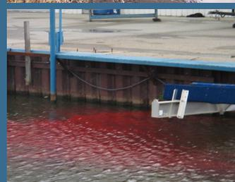
*The green dye in this picture confirmed that an illicit discharge was occurring through this storm water outfall along the Clinton River. The dye was put into the sewer cleanout from a facility a half mile away indicating the restroom waste travels directly to the river. The red dye confirmed this marina was discharging sanitary wastewater directly into Lake St. Clair.*
